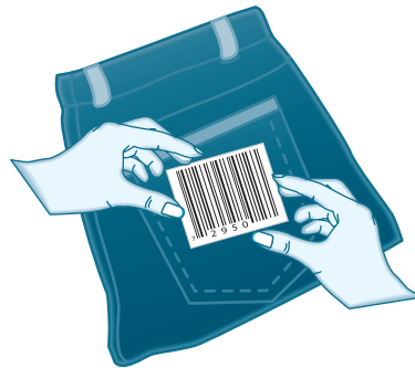
Bar codes are attached to the clothing to track it as it is assembled, washed, and prepared for shipment.
